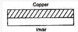
Diagram is to show how the given strip bends and cools. Due to heating the copper bends more than invar due to high coefficient of linear expansion of copper.
