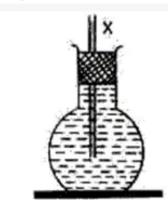
The level will rise above X when the flask is kept in hot water bath because the water in the flask will heat up and expand in volume thus raising the level of water in the tube above X
