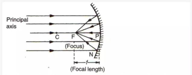
The parallel beam of light on reflection by a concave mirror converges at a point on the principal axis, midway between pole and the centre of curvature. This point is called principal focus
