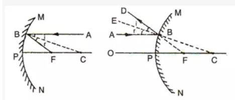
Let's assume the aperture of the mirror to be very small. Let a ray AB of light parallel to the principal axis be incident on the concave mirror at B. the ray makes the angle of incidence, i with the normal BC at B, C being the centre of curvature of the mirror. The ray is reflected along BF with angle of reflection, r so that
