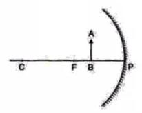
A light ray, parallel to the principal axis, coming from a point on object AB is reflected from the surface of the mirror, it passes through the principal focus and the other ray striking normally to the mirror reflects back and passes through the centre of curvature. These two reflected rays, when produced backwards, coincide at a point where the image is formed. The image, A'B' is virtual, erect, and magnified in size.
