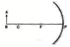
A light ray, parallel to the principal axis, coming from a point on object AB is reflected from the surface of the mirror, it passes through the principal focus and the other ray passing through the centre of curvature strikes the mirror normally i.e. 90 degree. Hence it will reflect back. These two reflected rays coincide at a point between F and C, where the image is formed. The image, A'B' is real, inverted, and diminished in size.
