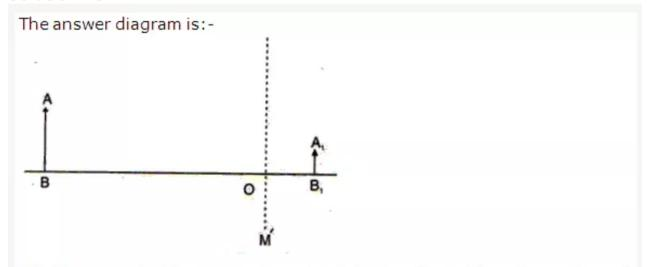
A light ray coming from a point on object AB is reflected from the surface of the mirror. When this ray is produced backwards, it passes through the principal focus and the ray which traces its incident path after reflection, when produced backwards, passes through the centre of curvature. These two reflected rays coincide at a point where the image is formed. The image, A'B' is virtual, erect, and diminished in size
