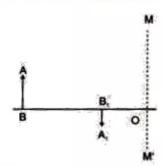
A light ray coming from a point on object AB is reflected from the surface of the mirror, it passes through the principal focus and the other ray passing through the centre of curvature strikes the mirror normally i.e. 90 degree. Hence it will reflect back. These two reflected rays coincide at a point where the image is formed. The image, A'B' is real, inverted, and diminished in size. The focal length was found to be 16 mm
