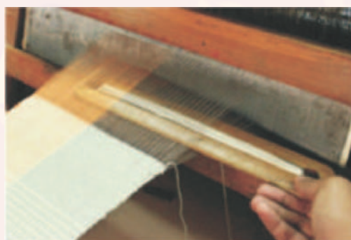
Fig 5.3: Picking with a Shuttle
