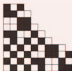
Fig 6.7: Faulty Repeat Unit - one complete repeat must be in a rectangular form
