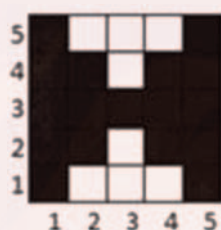
Fig 6.6: Wrong Design - Warp 1 and Warp 5 are forming loose floats
